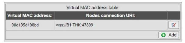
The VMAC is the virtual MAC address that is used under BACnet/SC to address data requests and responses that are sent or requested by the BACnet application. The virtual MAC address is then translated into the actual target URI in the BACnet/SC data link using a table and the data is then sent to the respective node via this URI.
