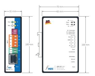
Specifications Power consumption: 1,7 watts Weight: 250 grams Dimensions: height: 100 mm, width: 30 mm, depth: 70 mm (incl. DIN top-hat rail adapter) Ambient temperature: 0...45°C, 23...113°F Ambient humidity: 20...80 per cent relative humidity, non-condensing Assembly: DIN top-hat rail TS35 in accordance with EN 60715
